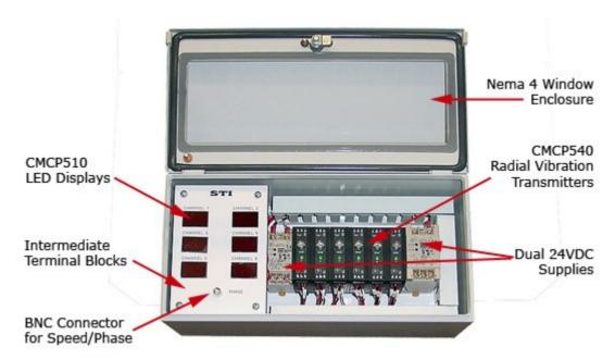
The STI System for each Unit was provided in a Nema 4 painted steel enclosure with window, bright Red CMCP510 LED Displays for each channel along with a BNC connector for Phase/Speed. As each CMCP540 Transmitter is provided with a BNC Buffered Output connections for balancing equipment are very straight forward. A complete wiring drawing was provided as part of the package in AutoCAD.
